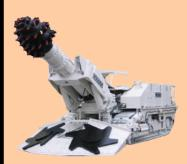
This machine makes roadways underground. It works like a big corkscrew, drilling through the coal. It is electrically powered and plugged into a gate end box.
