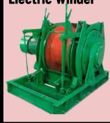
Electricity powers the winding engine, which lifts miners and coal in and out of the coal mine. An emergency winder is available if it breaks down. It is operated on the surface by mains electricity.
