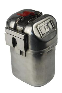
Miners wore a self-rescuer on their belts, and this was a compulsory piece of safety equipment. If there had been a fire or explosion, carbon monoxide is one of the gases produced and cannot be seen or smelt and can be fatal if breathed in. When a self-rescuer was worn, any carbon monoxide in the air is changed to carbon dioxide, which is breathable. The air breathed through the selfrescuer usually could keep a miner alive for 30-40 minutes.
